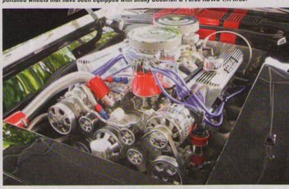
Displacing 490 ci and producing over 700 hp, this Shelby inspired engine features Demon carbs, MSD ignition Scat crank and rods. Edelbrock aluminum heads and much, much more.
